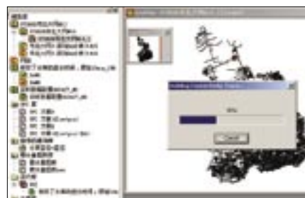
Isolated pipes and nodes could be deleted after connectivity tracing and confirmation of the results in the GIS.
