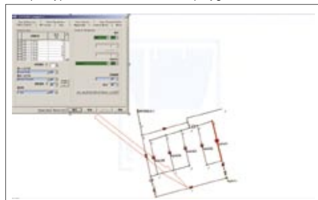
PRV control was used as valve control for the reservoir inflow.
